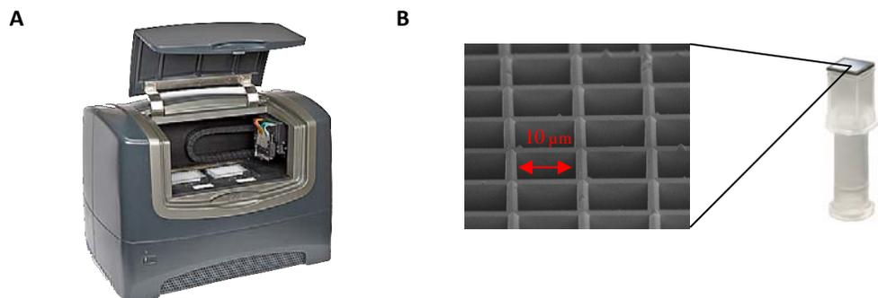
efficient mixing and transport of target molecules to the immobilized probes. Figure 1B shows an electron micrograph of the silicon chip which is fixed to a plastic tube to form a TipChip.
